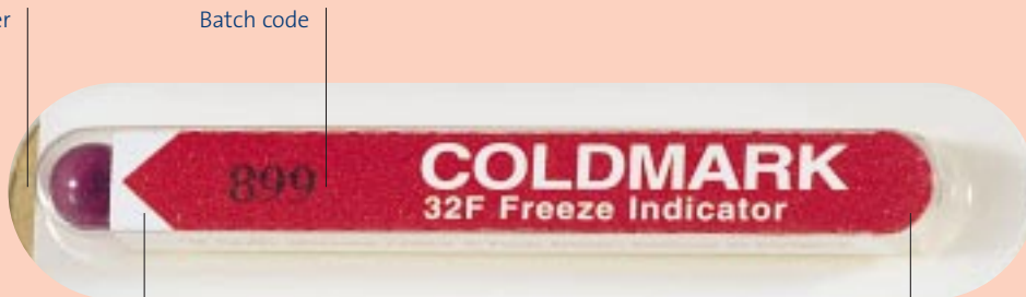
A clear colourless bulb indicates no exposure at or below response temperature
