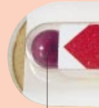
Violet indicates exposure at or below response temperature
